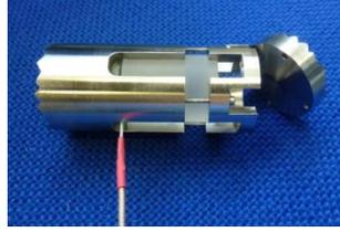
Fig. 1: INRiM's prototype of ultrasonic densimeter.
