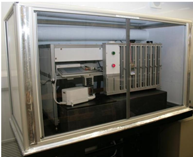
*Figure 3: Chamber used for filter weighing at NPL*
