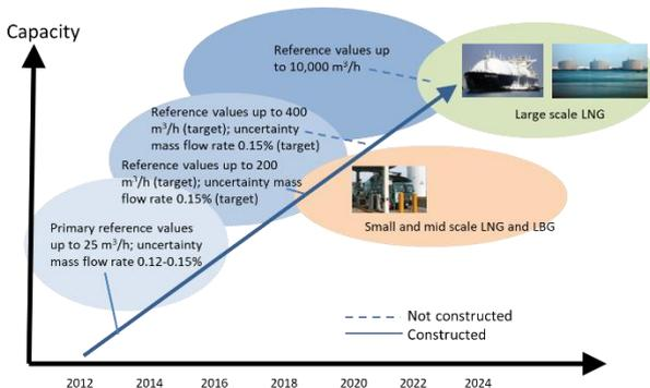
**Figure 1:** Roadmap for traceable LNG flow meter calibrations. LBG denotes liquefied biogas.
