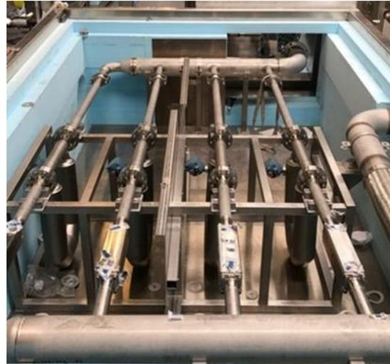
Figure 4: working standards, a set of Coriolis mass flow meters.
