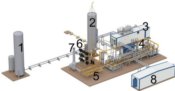
Figure 3: The Cryogenic Research and Calibration facility: 1) Liquid Nitrogen (LiN) storage tank, 2) cryogenic liquid storage tank, 3) primary Standard (PSL) for mass flow utilizing the gravimetric method to calibrate the Coriolis mass flow meters in the PSL, 4) Meter under Test (MuT) section, 5) working standards, a set of Coriolis mass flow meters, 6) heat exchangers and pumps, 7) Nitrogen (N<sub>2</sub>)-warmer and 8) control room.
