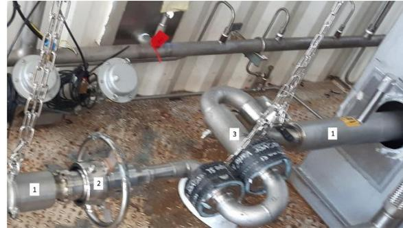
**Figure 6:** Dry-break coupling in the primary LNG mass flow standard. Components indicated are: filling pipe (1), dry-break coupling (2), and the swivel pipe (3).
