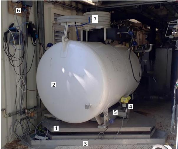
**Figure 3:** The LCS, balance, and weighing vessel of the primary LNG mass flow standard. Components are: balance (1), weighing vessel (2), floor board (3), actuators (4), tank frame (5) LCS control system (6), and calibration weights (7).
