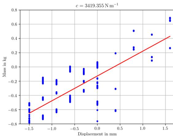
**Figure 5:** Actual displacements enforced by the LCS (top; negative is lowering) and corresponding measured mass deviations (bottom). From the linear regression a stiffness value of the filling pipe and other tank appendages is estimated.
