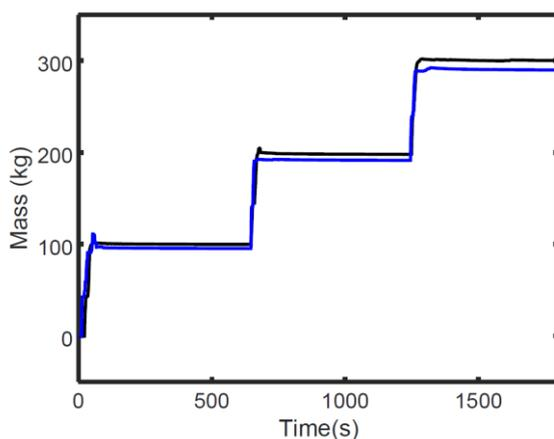
**Figure 4:** Mass readings as a function of time with LCS on (black) and LCS off (blue).
