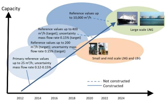
**Figure 1:** Roadmap for traceable LNG flow meter calibrations. LBG denotes liquified biogas.
