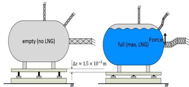
**Figure 2:** When the tank is loaded during the filling process of the weighing tank, a resulting force is created due to the lowering of the tank and the stiffness of the filling pipe (and other appendages).
