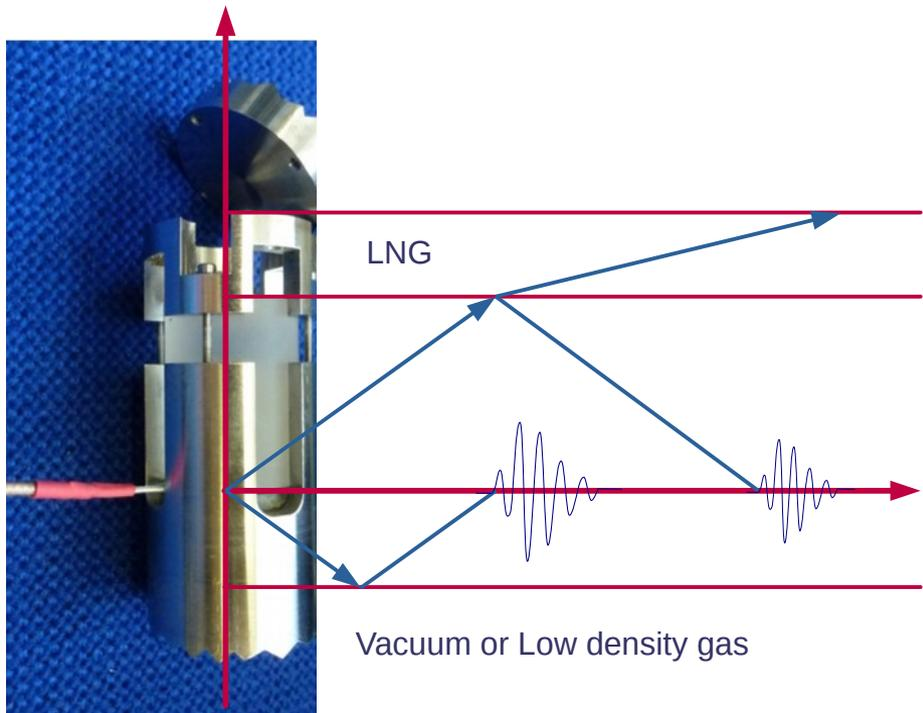
INRiM's pycnometer (prototype I) for cryogenic density measurements
