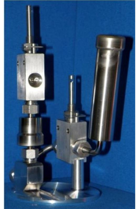
INRiM's pycnometer for cryogenic
