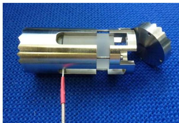
**Figure 5** – INRiM's sensor for the simultaneous measurement of the density and speed of sound of a fluid based on the determination of the acoustic impedance of the sample.
